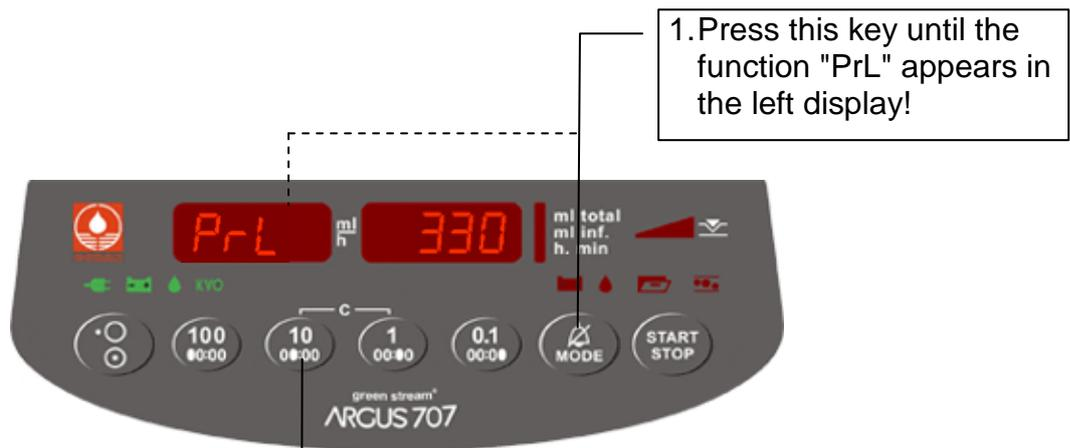
2. Press this key and the new occlusion pressure limit appears in the right display! (Limit is set according to above mentioned formula). The neonatology mode is now activated. If no key is pressed within 5 seconds (programmable) the display changes back to the basic position!
