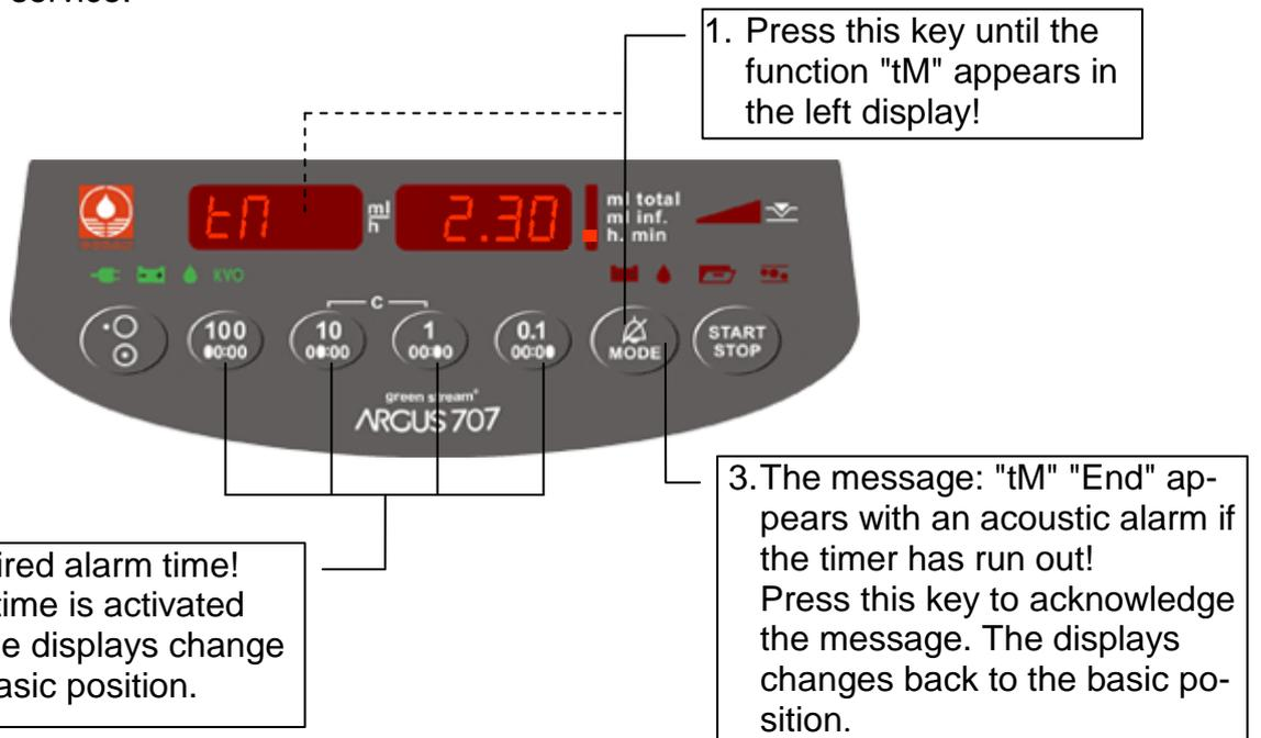
The remaining time can be checked by selecting the function timer "tM".
