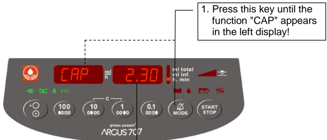
2. The right display shows the battery running time in hours and minutes (e.g. 2 h 30 min).
