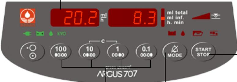
The diagram shows the control panel of an ARGUS 707 infusion pump. The display shows a current flow rate of 20.2 ml/h and a remaining infusion time of 8.3 h. The panel includes several buttons: a power button, a numeric keypad (100, 10, 1, 0.1), a MODE button, and a START/STOP button. Callouts provide the following instructions:
