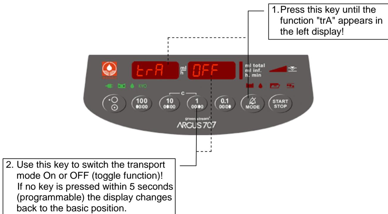
In run mode, if this function is turned on, the message "trAn" "SPOR" is blinking alternatively with the infusion rate display.
