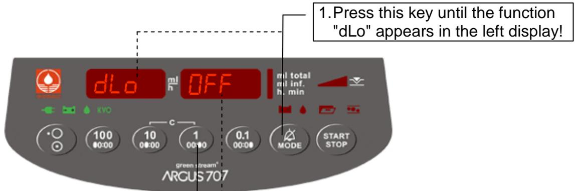
2. Use this key to switch the data lock ON or OFF (toggle function)!
