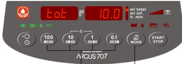
5. Use these keys to enter a new bolus volume (e.g.10.0)! If no key is pressed during 5 seconds (programmable), both displays change back to the basic position!
