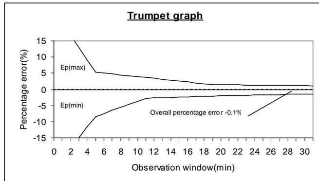
Test I in the first two hours of the test period of 24 hours at 25 ml/h (initial period)
