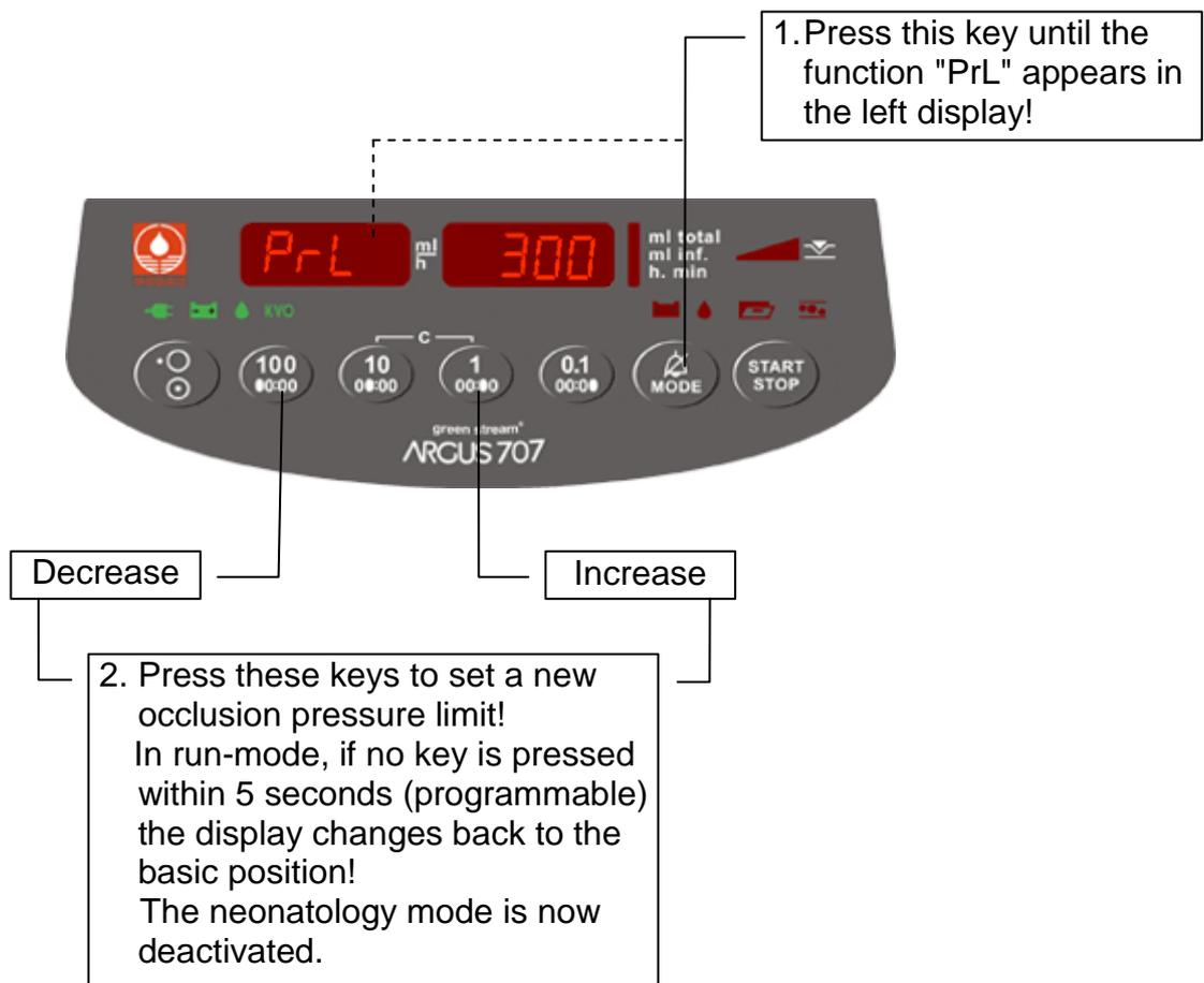
**CAUTION :** Opening the door, turning OFF the pump or the occlusion alarm will automatically deactivate the neonatology mode.
